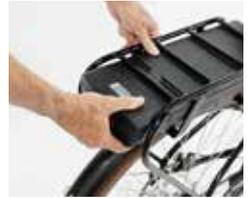
To be able to use the electric motor, the battery must be mounted by sliding the fully charged battery forward into the battery holder.
