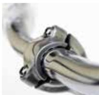
6. Make sure the seat is tight enough so that you can't twist it out of alignment. Pull the seat clamp handle away from the seat post and slide the seat up or down to adjust it. Move the clamp handle inward toward the seat post so it is held tight by the clamp.
