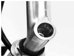
If need be, the angle of the handlebars may be positioned to your personal preference. Loosen the front 2 bolts on the front stem plate and angle the handlebars to your liking, then securely tighten the 2 bolts on the front stem plate. Make sure that, when tightening, there is even spacing between the top and bottom bolts to ensure maximum stability.
