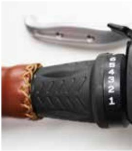
Your Pedego is equipped with 7 speeds on the City Commuter and the Interceptor. The first gear is for easier and uphill pedaling, and the last gear is for maximum speed on level or downhill terrain. Change gears only while pedaling. The rear wheel contains seven chain sprockets. When the chain is around the largest sprocket, you are in 1st gear, or the lowest gear. The high gear will have the derailleur positioned so that the chain is directed around the smallest gear.
