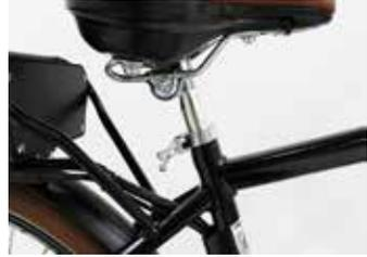
If necessary, tighten the clamp by twisting the clamp handle clockwise while in the un-clamped position. Then, fold the handle in toward the seat post. This should require a fair amount of force to ensure the seat post is held tight. If necessary, the clamp can be further tightened with an allen key when in the clamped position. Make sure the seat is not set with the vertical maximum height marks above the clamp.
